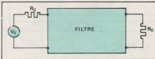
$$N = \frac{0,693 + 0,115 \alpha_{\min}}{\log_e \left[ \frac{f_a^2 - f_c f'_c}{f_a (f_c - f'_c)} + \left[ \frac{(f_a^2 - f_c f'_c)^2}{f_a^2 (f_c - f'_c)^2} - 1 \right]^{1/2} \right]}$$
